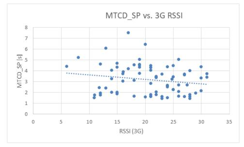
Figure 8-13 MTCD for Smartphone-type devices in the A role vs. averaged RSSI per location.
