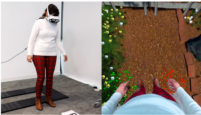
Figure 3 – Video-based avatars. Left : A person wearing an HMD with an attached egocentric camera, so that her body is captured from the camera, segmented, and integrated within a virtual environment. Right : The virtual environment as perceived by the HMD user, with she can see her own body.
